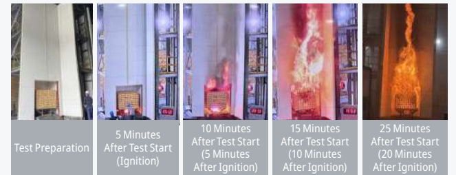
Testing scenes of fire safety performance of Aekyung Chemical's semi-noncombustible insulation material for building exterior finishing systems
